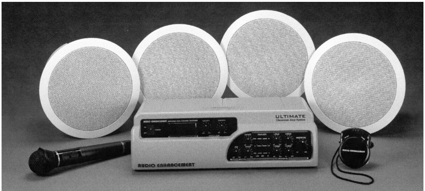
FIGURE 1. Photograph of an infrared sound-field amplification system; the teacher wears a wireless microphone transmitter, and the speech is sent via light waves to an amplifier and loudspeakers. The four circular loudspeakers are designed to be mounted, in a distributed fashion, in a drop ceiling. The handheld microphone is a pass-around microphone for the pupils to use (to facilitate auditory self-monitoring of their own speech as well as to enable the talker to be heard by all students in the room). The small, black, circular infrared transmitter is worn by the teacher. (Photo courtesy of Audio Enhancement)
