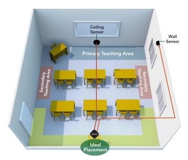
Area in green is a good balance of sound distribution and viewing angle. Additional ceiling or wall sensor may be required.
