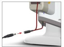
2. Verify cables are fully inserted into USB hub.
